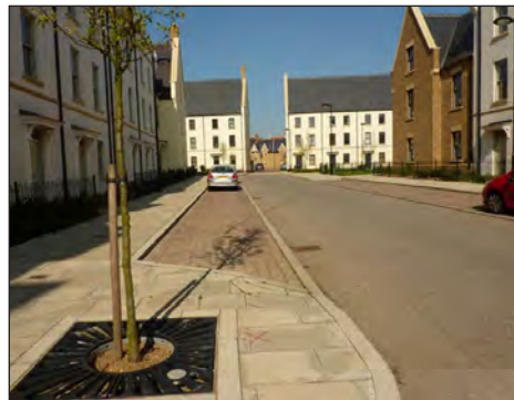
On-street parking designed into the street scene and identified by changes in surface material
