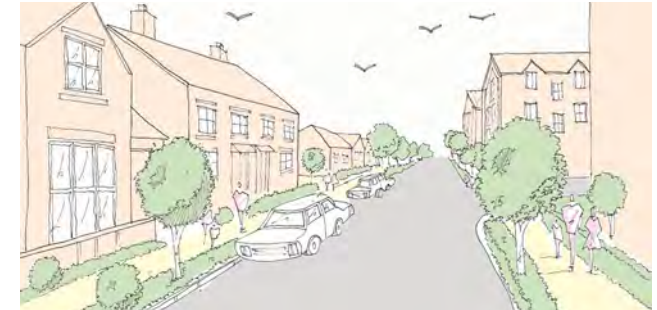
Figure 66: Improve on street parking by designing bays that are broken up by planting, rain gardens and streets trees.
