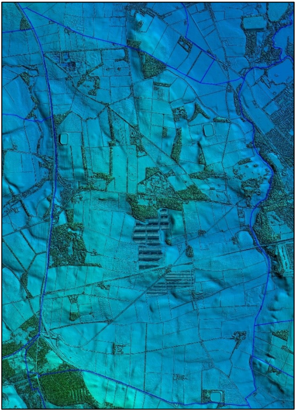
Figure 8.2.1 Surface height model from LIDAR (APGB, via Parish Online)
