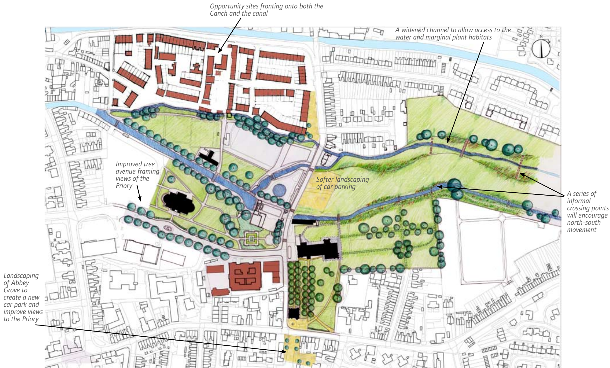
Outline landscape plan showing footpaths, crossings and desired tree layout. New housing is suggested for key opportunity sites
